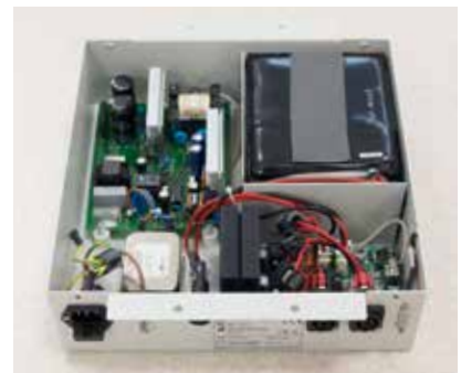
Heavy-duty mobile battery powers the unit for up to 8 hours of use
